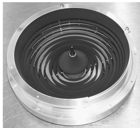
FIG. 9. Outer ESA electrode with fins. Particles from the conversion surface always hit the fins on a face with no direct line of sight from the impact point to the ESA exit. The complete assembly is 298 mm in diameter.
